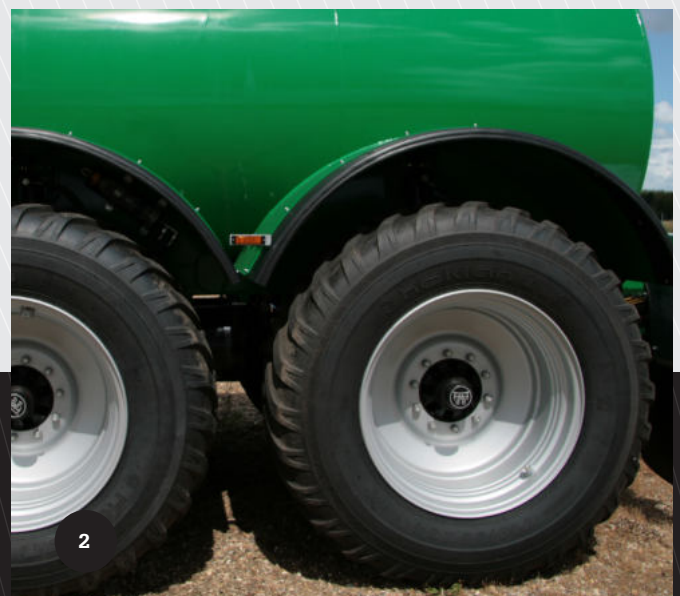
The large wheels reduce rolling resistance.
