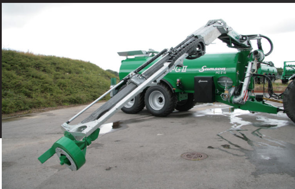
Pump tower with telescopic arm
