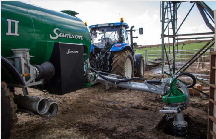
Direct filling from underground storage of slurry
