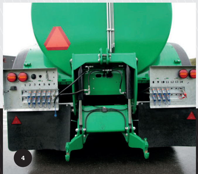
Hydraulic couplings are located where they are easily accessible.
