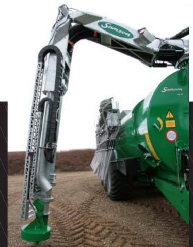
The new pump tower is more flexible, making the operation of the pump tower easier when emptying covered slurry lagoons where you navigate through small openings, or when emptying underground slurry stores.
