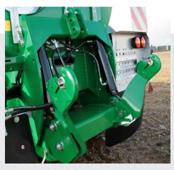
The new lift can lift up to 9 tonnes in a horizontal position and deliver a pressure of 5 tonnes.
