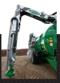
The new pump tower is more flexible, making the operation of the pump tower easier when emptying covered slurry lagoons where you navigate through small openings, or when emptying underground slurry stores.
