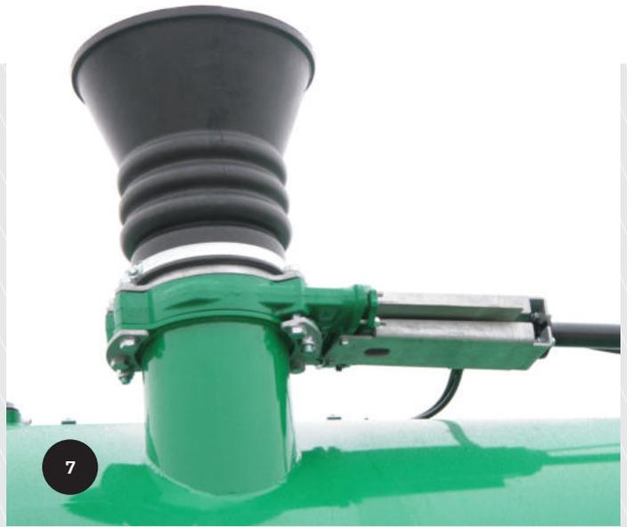
The funnel is closed using a hydraulic slide valve to avoid surges and soiling of the vehicle during transport.
