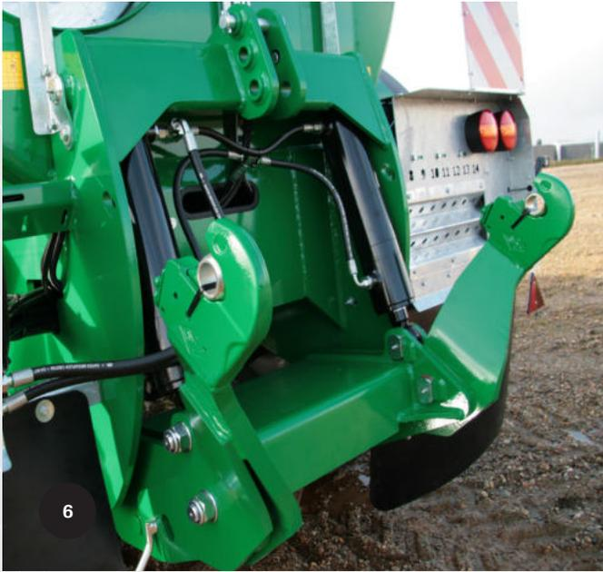
The new lift can lift up to 9 tonnes in a horizontal position and deliver a pressure of 5 tonnes.
