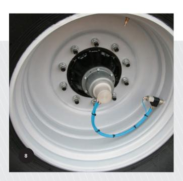
SAMSON AGRO's automatic tyre pressure regulation is a two-circuit system with shut-off valves in each wheel.
