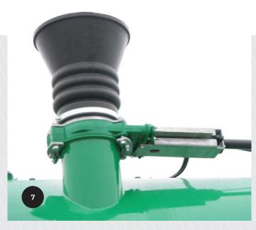
The funnel is closed using a hydraulic slide valve to avoid surges and soiling of the vehicle during transport.
