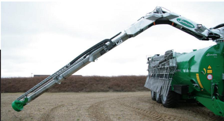
The pump tower is now more compact. The 6-inch reflux pipe is integrated into the pump tower. It now has a telescopic function giving it a longer reach.
