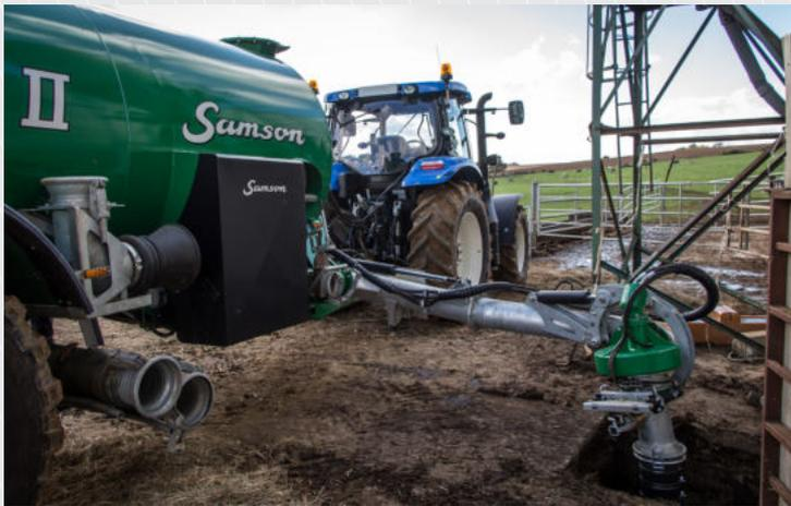
Direct filling from underground storage of slurry
