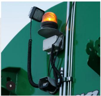
Rotor beacons are used as a warning to prevent slurry tanker overflow.
