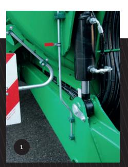
Drawbar suspension gives optimal driving comfort. The height can also be adjusted.
